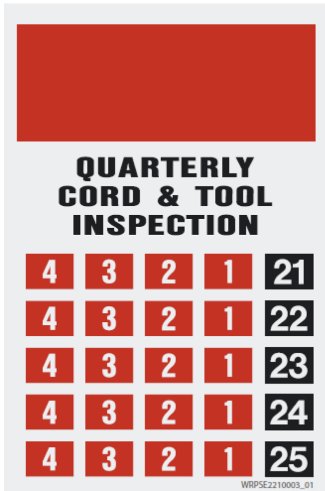
FIGURE D-3: QUARTERLY INSPECTION TAG EXAMPLE
