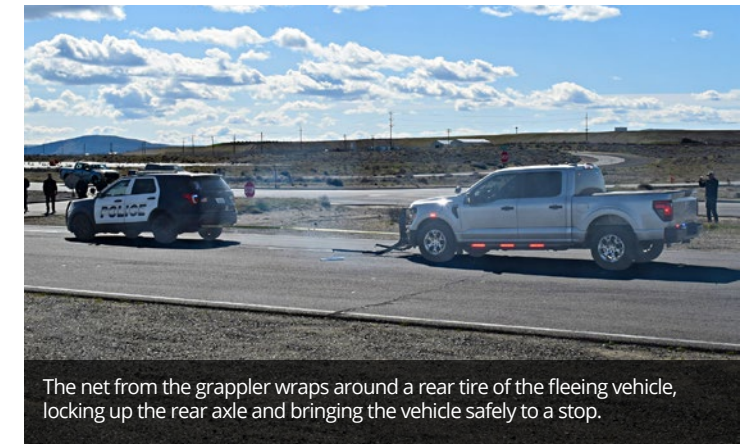
During a pursuit, the grappler is deployed from the front bumper of the patrol vehicle (the silver pickup in this photo).
