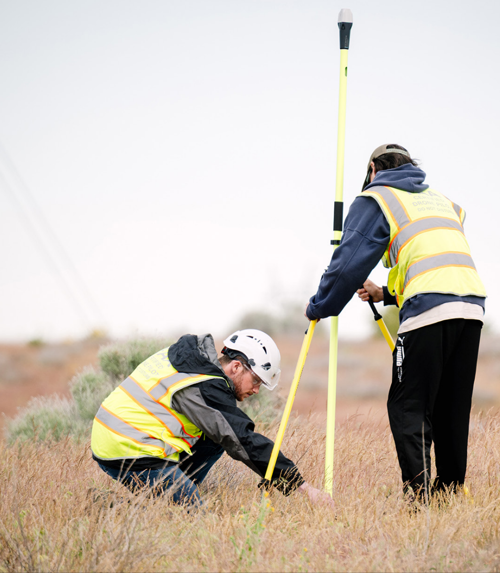
UAS pilots prepare for a lidar flight by setting ground control points which establish an accurate position for the flight's path.
