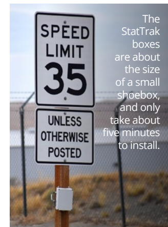
The StatTrak monitors can be mounted on any existing sign or pole and use microwave signals to measure the numbers of vehicles that pass by.
